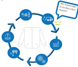
Packaging collected separately is taken to selection plants. After washing at 200°, the cooled, fluid paste is "reborn" in granular form, which can be given new shapes.
