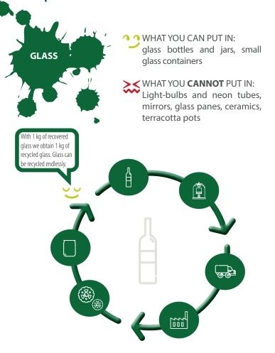
The glass collected, when deprived of its "false friends" (glass panes, ceramics, mirrors, etc.), arrives at the furnaces in the glassworks where it is melted at over 1500°. Using the appropriate moulds, it takes on new shapes and can be recycled endlessly!
